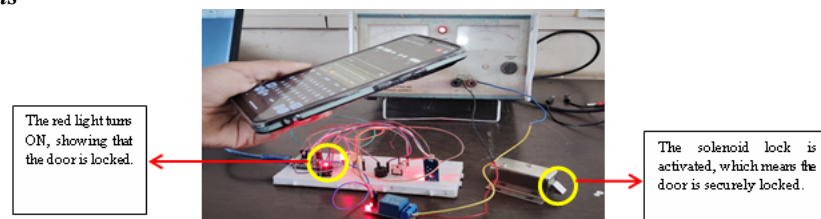
Figure no 3: Door locked condition (incorrect/no code)
